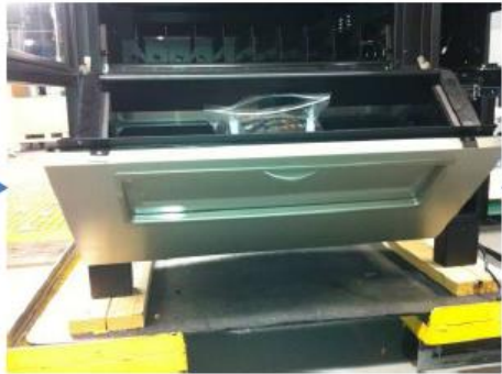
Bin pulled out to access bolts
